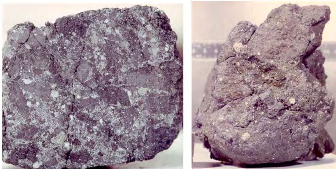
FIGURE 3.44 Examples of a polymict breccia on the left (sawn surface of sample 14306,21, about 6 cm across, NASA # S77-22103) and a regolith breccia on the right (sample 15299,0, the scale in background is in cm, NASA # S74-32566).
